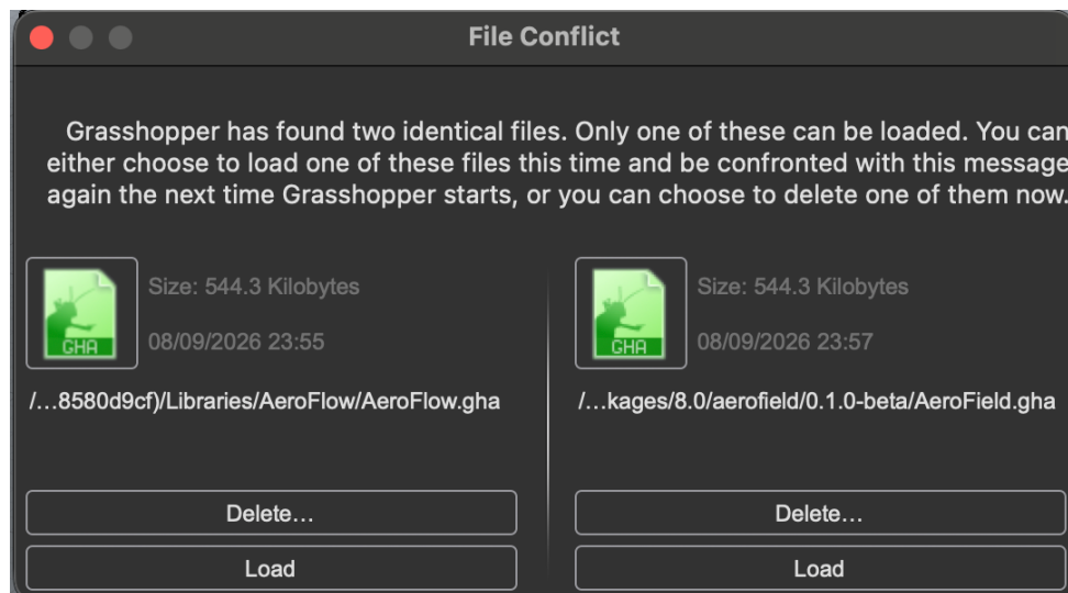
Figure 16.1: A duplicate assembly conflict. Keep the intended current installation and remove the other copy.
